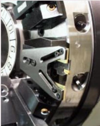
PULLEX feeds the bar within 1.5 - 2 seconds, to be compared with the job of a conventional Shortbar Feeder, which would take 10-15 seconds to execute the same operation.
